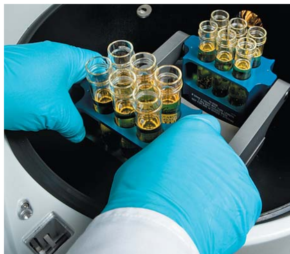
EZ-2 accepts a wide range of formats, including flasks, vials, tubes and microtitre plates.
